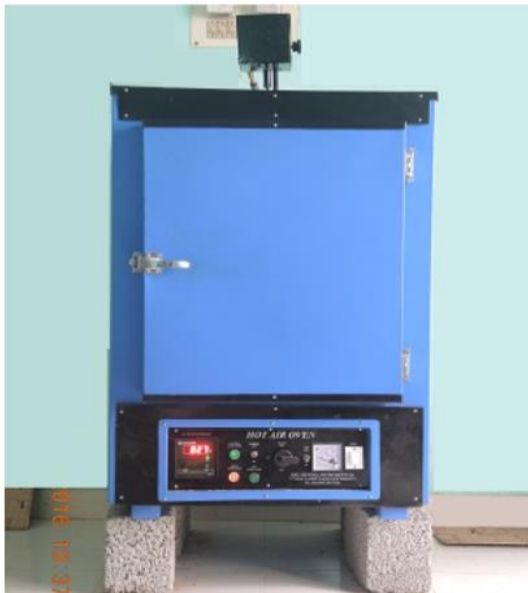
Bitumen Blending Oven
