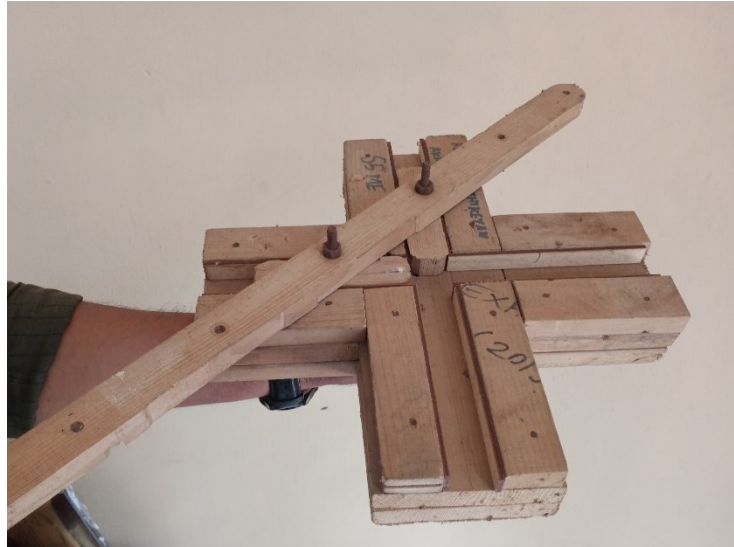
Figure 4: Model of an elliptical trammel mechanism used by Prof Antony J K for teaching Theory of Machines classes.
